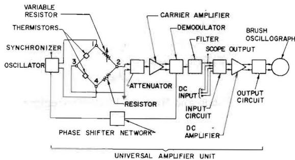
Fig. 3 Thermistor velocity-recording device
