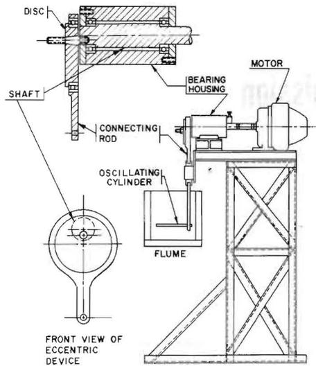
Fig. 2 Vibrating cylinder and flume apparatus
