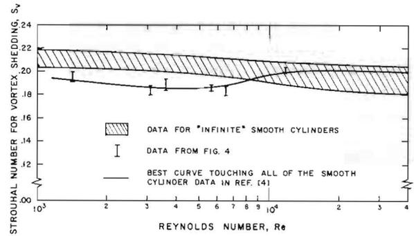
Fig. 6 Dependence of  $S_{V_0}$  upon  $Re$  for "infinite" cylinders and for present tests
