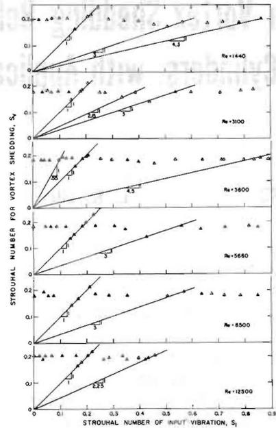
Fig. 4 Influence of cylinder frequency upon vortex frequency, 6 typical cases,  $A/D = 0.125$
