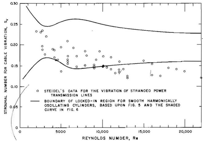
Fig. 7 Comparison present locked-in region with Steidel's transmission line data
