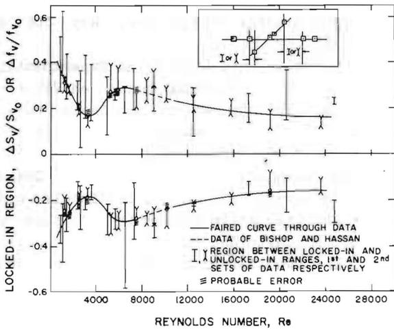
Fig. 5 Dependence of fundamental locked-in region upon Reynolds number,  $A/D = 0.125$
