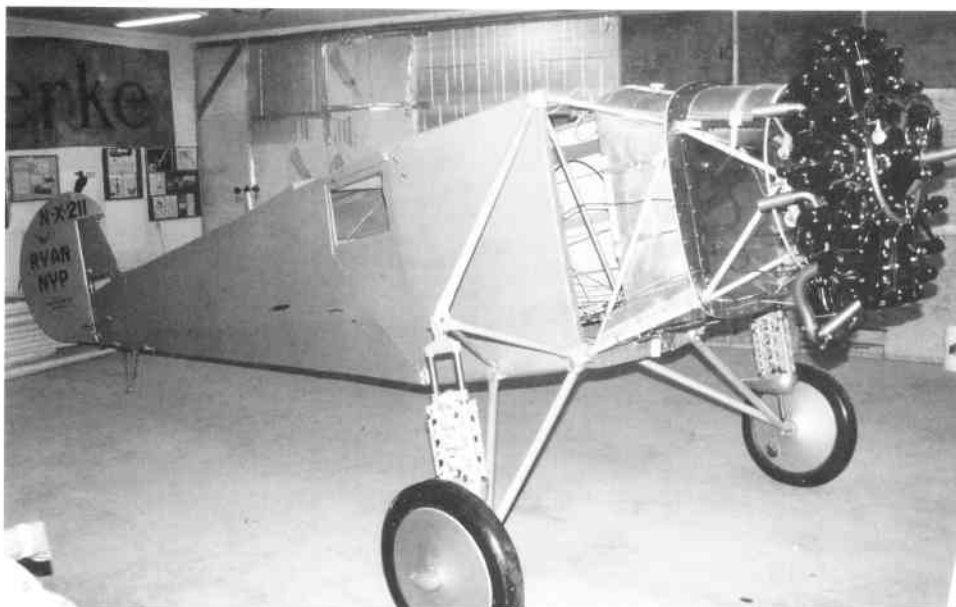
Spirit with fuselage covered and Wright J-5 installed and sitting on gear.
